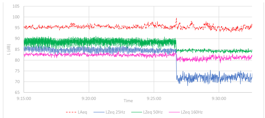
Figure 6. Loss-of-chaos signature simultaneously affecting the 25 Hz and 50 Hz bands during ISO 3744 [25] testing (single engine in operation).
