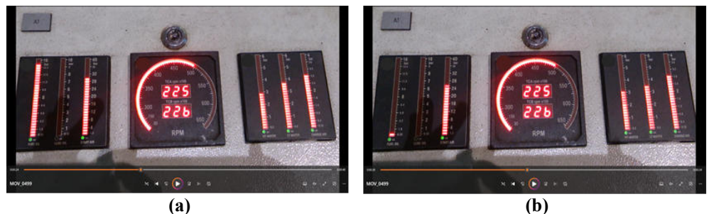
Figure 4. Engine control commands during testing according to ISO 3744:2010: (a) Fuel pressure at its near-maximum point (16 bar); (b) Fuel pressure at zero, 6 s later.
