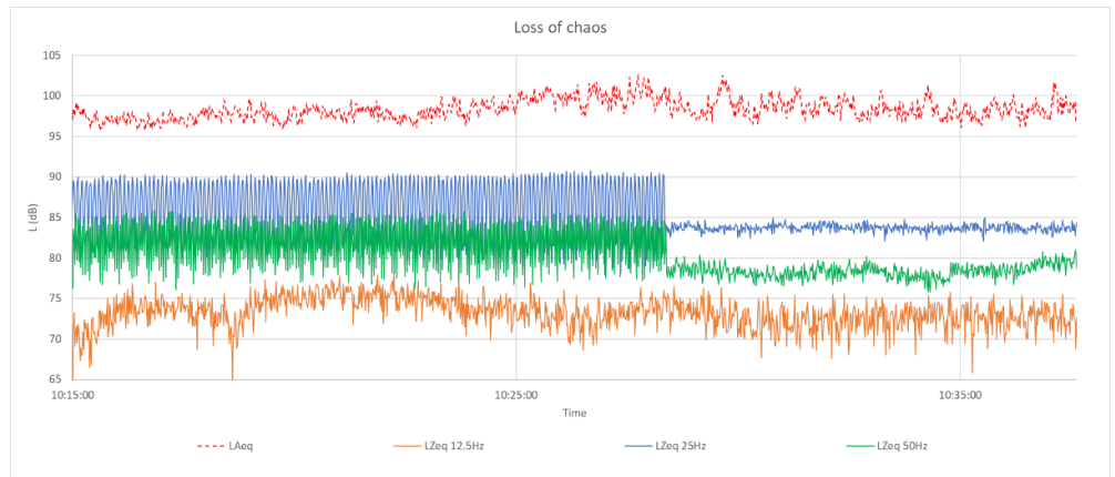
Figure 8. Loss-of-chaos signature simultaneously affecting the 25 Hz (blue) and 50 Hz (green) bands during ISO 3744 [25] testing (single engine in operation). Note: Sudden decreases of approximately 5 dB at 25 Hz and 50 Hz are observed.
