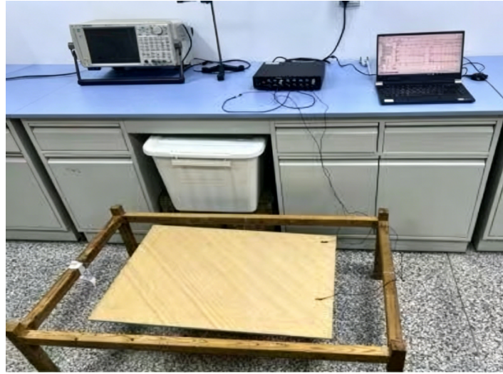
Figure 2. Measuring system with cross-suspension support and the positions of excitation and the accelerometer.
