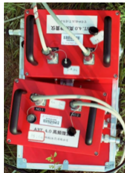
(b) High-frequency geological structure monitor
