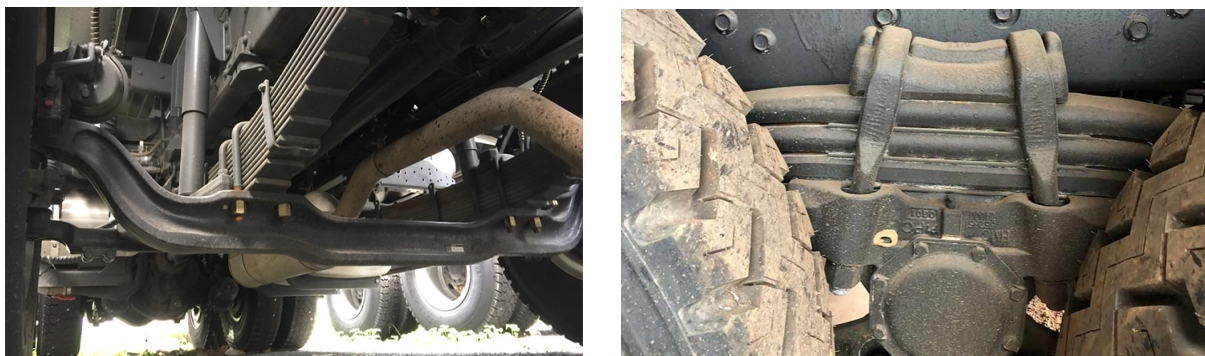
Figure 3. The front axle dependent suspension and the rear axle balanced suspension are features of 3-axle trucks.
