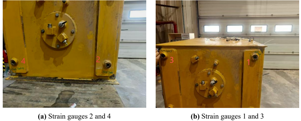
Figure 15. Actual placement position of strain gauges.
