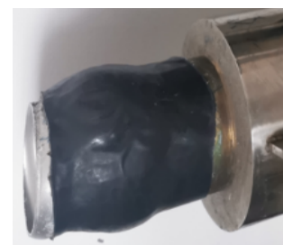
(c) Wrapped with heat-shrinkable tube.
