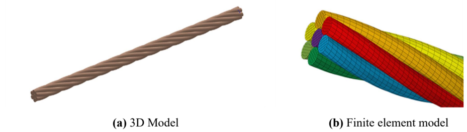
Figure 3. 3D and finite element models of the dropper.
