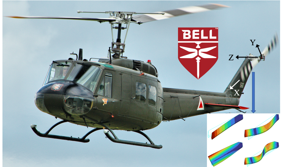
Figure 1. Bell UH-1H [17] showing the XYZ coordinate system of our tail rotor.
