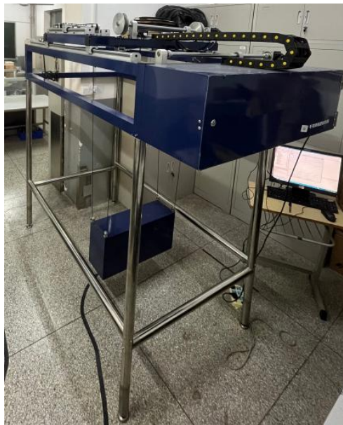
Figure 8. A small-scale RTG model, consisting of an angle detection system, a motion control system, and a monitoring system.
