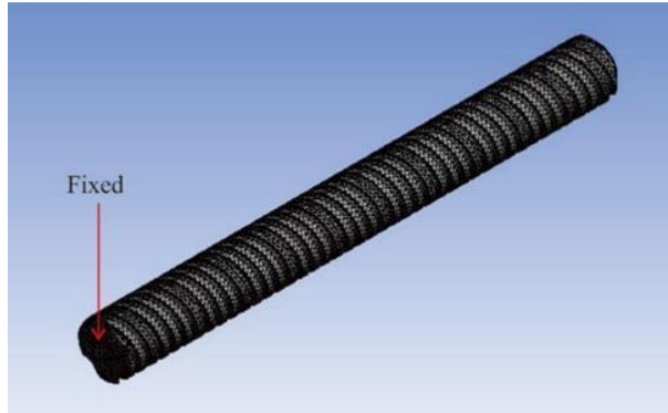
Figure 16. Finite element model and boundary constraint of the compensator.
