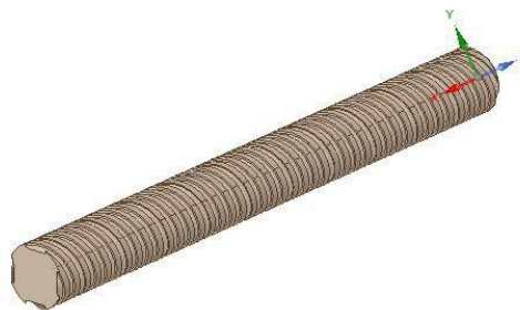
Figure 15. 3-D model of the slack adjuster compensator.
