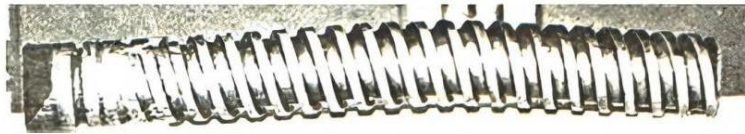
Figure 2. Bent tread compensator of the air braking system [17].
