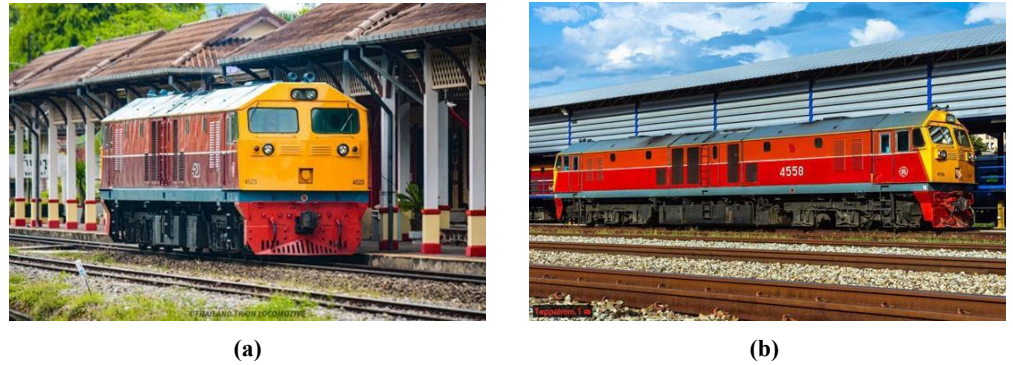
Figure 4. The diesel-electric locomotive series GEA 4523–4560 used in the paper (a) The diesel-electric locomotive series GEA 4523 for passenger and freight traffic [24]; (b) The diesel-electric locomotive series GEA 4558 for passenger and freight traffic [25].
