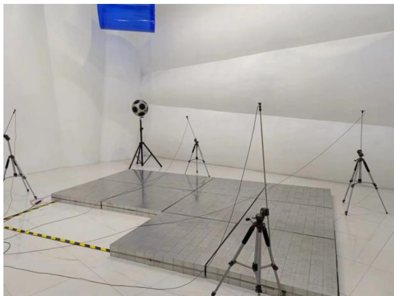
Figure 16. Measuring the sound absorption coefficient of SAS in a diffuse sound field using the reverberation chamber method.
