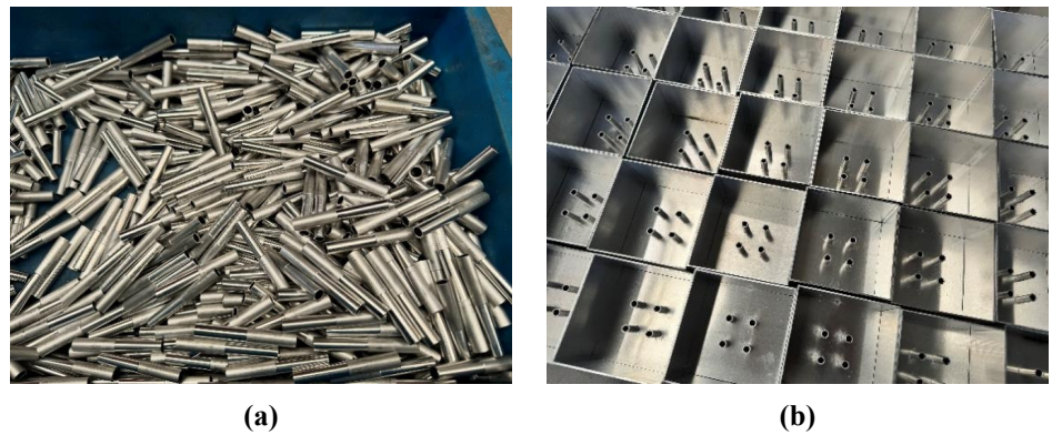
Figure 8. The manufacture of SAS. (a) Inserted ducts; (b) Cavities equipped with inserted ducts.
