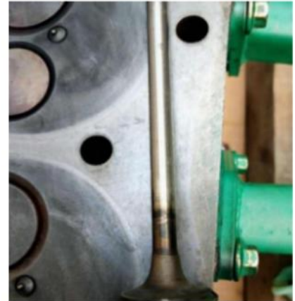
(b) Burning of exhaust valve spindle.
