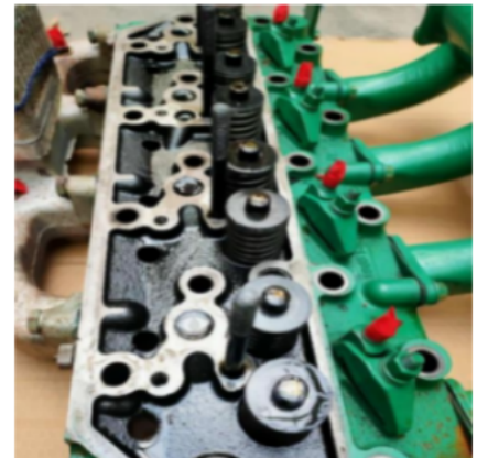
(d) Cylinder head valve assembly of diesel engine.
