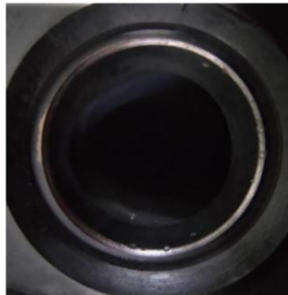
(a) Pitting corrosion of exhaust valve seat.
