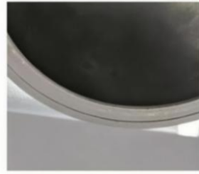
(c) Excessive wear of cylinder liner (+0.5 mm). (d) Cylinder wall damage condition.
