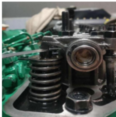
(c) Excessive clearance of exhaust valve.
