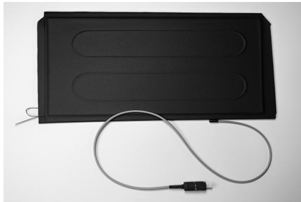
Figure 3. Sample composite plate with integrated fiber optic sensor.
