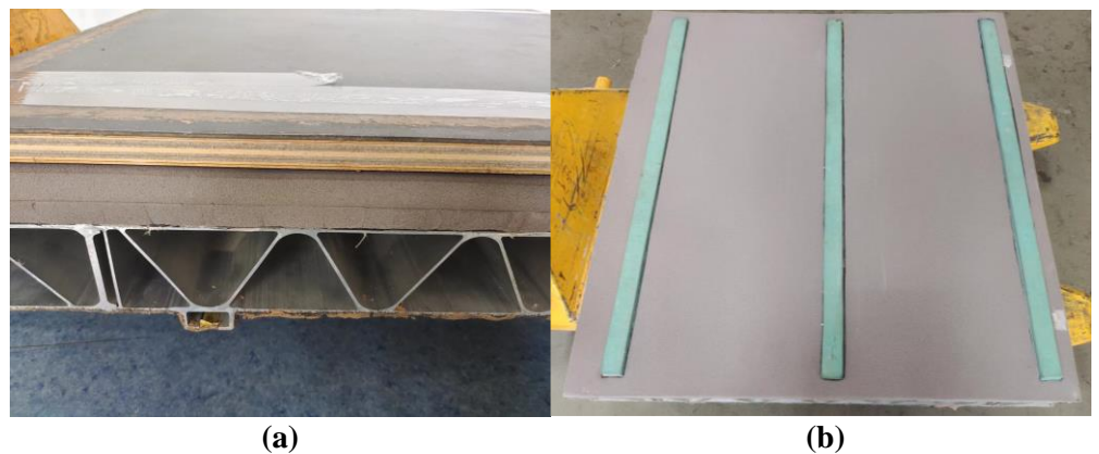
Figure 13. Floor structure diagram. (a) Cross-sectional photography; (b) Distribution diagram of wooden support structure.
