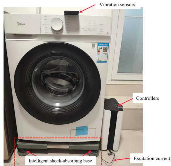
Figure 12. Dynamics test of intelligent vibration damping base of drum washing machine.
