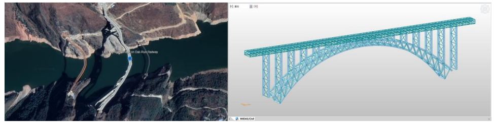
Figure 14. The location of Lancang River Bridge on Dali-Ruili Railway and the modeling of the main span.
