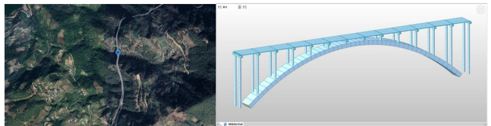
Figure 10. The location of Feilong Bridge and the modeling of the main span.
