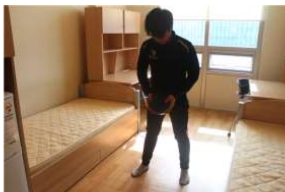
Figure 12. Floor impact noise measurement using rubber ball.
