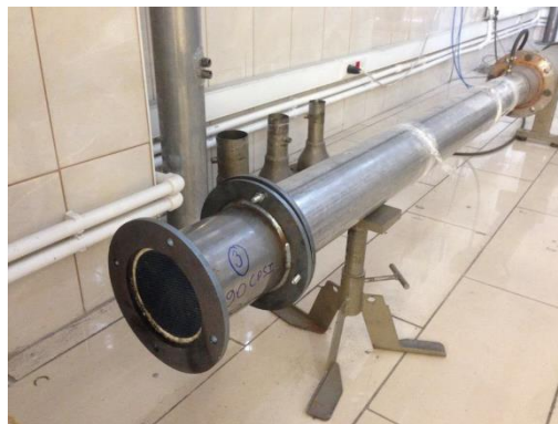
Figure 4. Pressure test setup.
