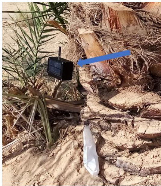
Figure 2. The recording of red palm weevil sounds using an acoustic sensor installed inside a date palm tree.
