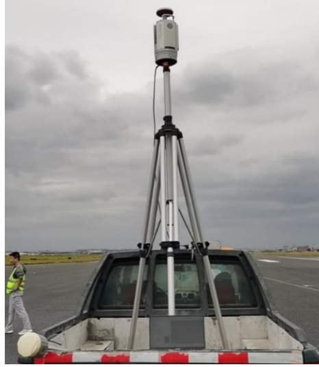
Figure 2. Three-dimensional laser point cloud static measurement.
