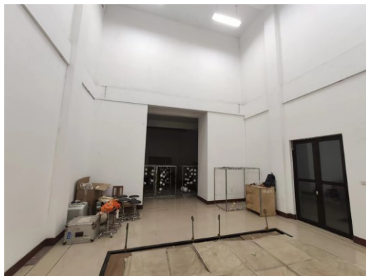
Figure 1. The photo of the reverberation room.
