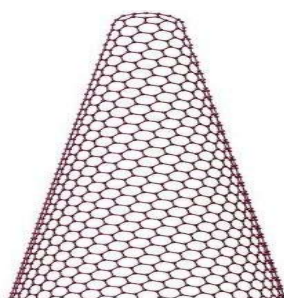
Figure 3. The structure of carbon nanohorn [47] .
