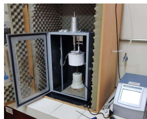
Figure 5. Cavitation test equipment.
