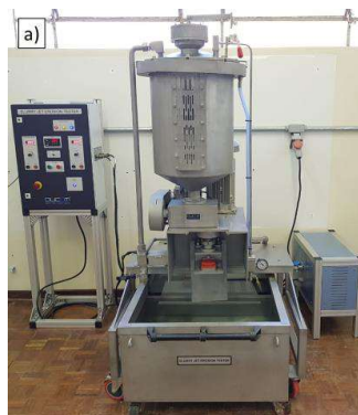
Figure 6. DUCOM Mud Jet Equipment used in erosive wear tests; (a) General image of the equipment.
