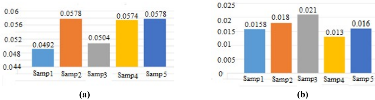
Figure 8. Variation of the linear mass of the fibers. (a) Stems; (b) Roots.
