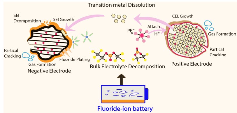
Figure 6. Schematic presentation of electrolyte degradation of a fluoride ion battery.
