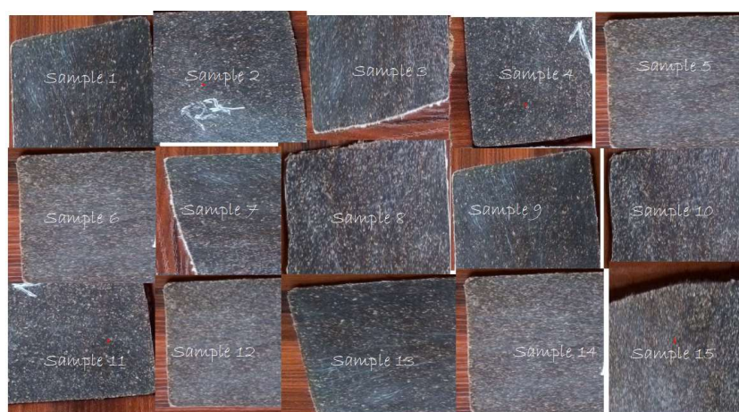
Figure 5. Rice husk-based reinforced particle board.
