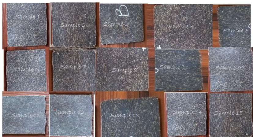
Figure 4. Bagasse-based reinforced particle board.
