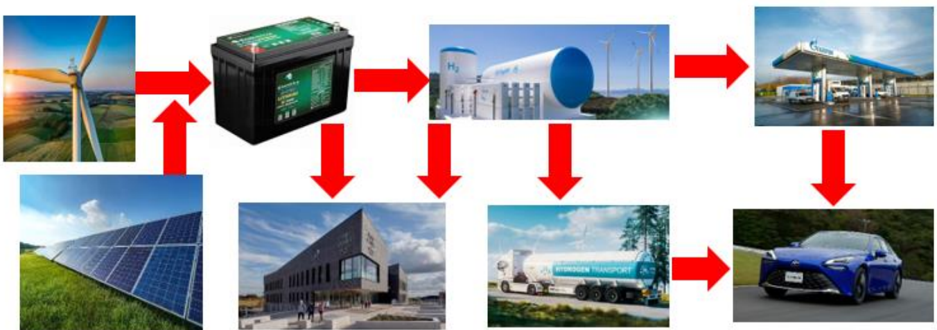
Figure 3. Diagram of the supply chain for a green private wire community starting on left with solar/wind charging a battery that feeds buildings and powers an electrolyser /hydrogen store leading to hydrogen for shipping plus vehicle refuelling and buildings energy.
