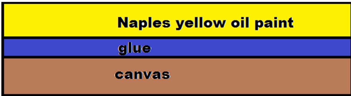
Figure 3. Schematics of three layers painting on canvas.
