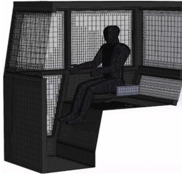
Figure 1. Diagram of meshing of the air-conditioned cabin.
