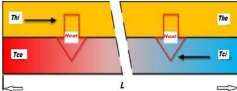
Figure 2. Schematic representation of Counter-Flow Heat Exchanger<sup>[5]</sup>.
