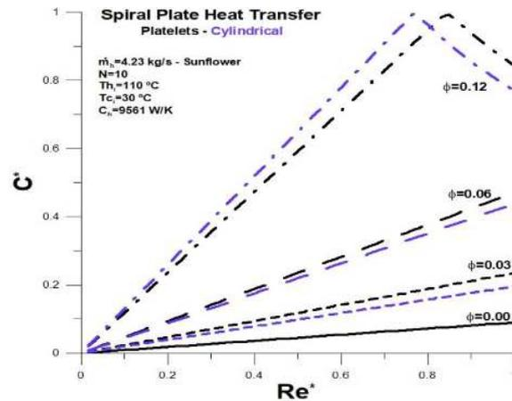
Figure 4. Relationship between heat capacities versus Reynolds number.
