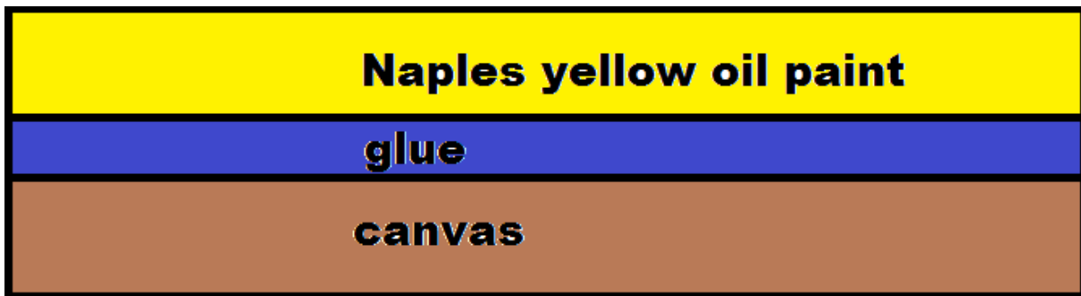
Figure 3. Schematics of three layers painting on canvas.
