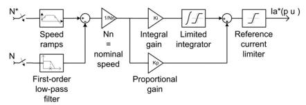
Figure 5. Traction electric motor speed regulator block.
