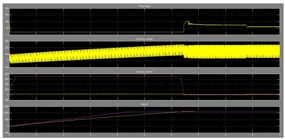
**Figure 14.** Temporal changes of the ignition angle of the rectifier thyristor, voltage and armature current of the ŽS 444 series locomotive electric motor in light passenger trains.
