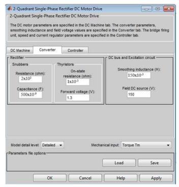
Figure 10. Layout of the thyristor rectifier table dialog.
