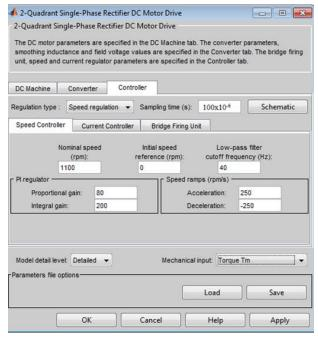
**Figure 11.** Layout of the speed controller table dialog.
