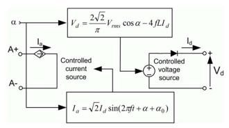
Figure 7. Single-phase thyristor rectifier block.
