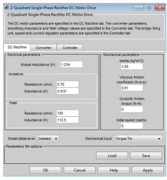
Figure 9. Layout of the dialog table of the drive electric motor of direct current.
