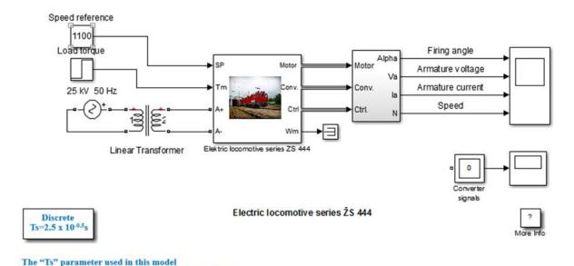
**Figure 3.** Structural scheme of the model of the 444 series electric locomotive in Matlab-Simulink during speed control.
