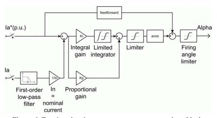
Figure 6. Traction electric motor armature current regulator block.
