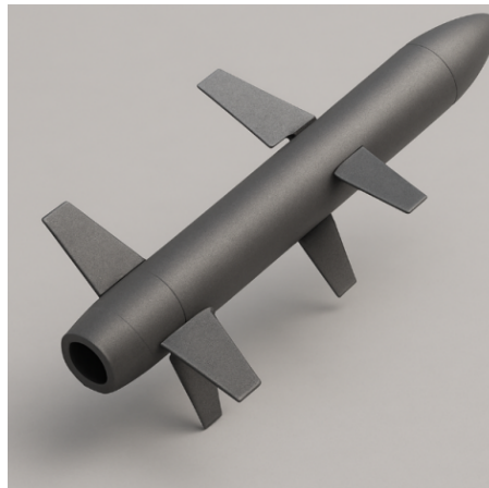
Figure 3. Small-Scale Maneuverable Solid Rocket with Canards and Winglets.
