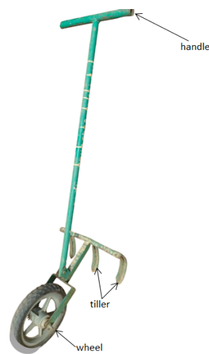
Figure 1. Hand tilling device after construction.
