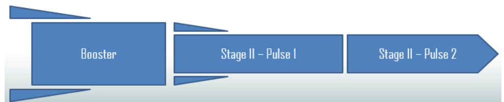
Figure 13. Selected propulsion system schematic configuration: Two-stages motors with the second stage based on two pulses.
