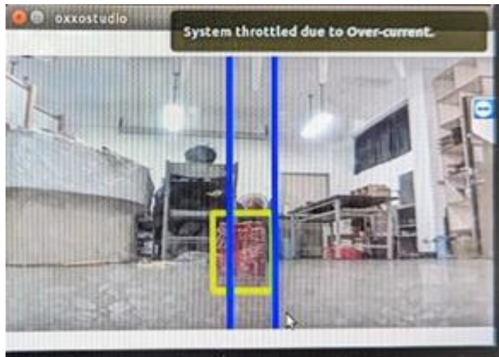
Figure 20. Schematic diagram of cleaning robot tracking using CSRT (yellow box).
