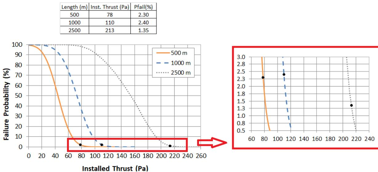
**Figure 1.** Failure probability curves for tunnel lengths.
