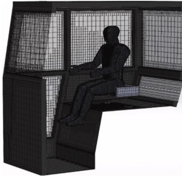
Figure 1. Diagram of meshing of the air-conditioned cabin.
