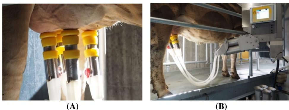
Figure 2. Milking parlor. (A) Milking cup with SSL teat liner; (B) multiLactor milking machine (Siliconform, Germany).
