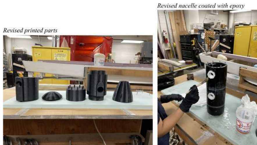
Figure 15. Revised design of nacelle coated with epoxy and its parts.
