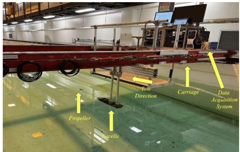
Figure 17. Photograph of the prototype turbine during the towing tank experiment.
