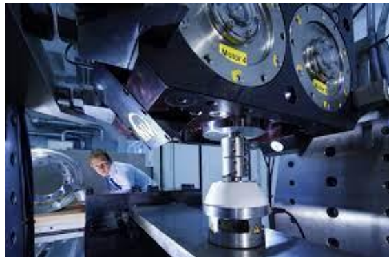
Figure 1. Active vibration control.
