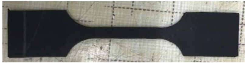
Figure 1. Neoprene rubber sandwiched with a bi-directional carbon fabric composite specimen.
