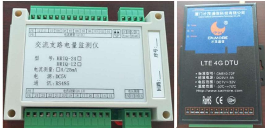
Figure 1. Data acquisition equipment.
