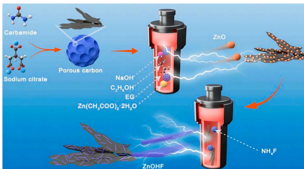
Figure 6. Schematic of the synthesis routes of ZnOHF-embedded N-doped porous carbon nanocomposite [45] .
