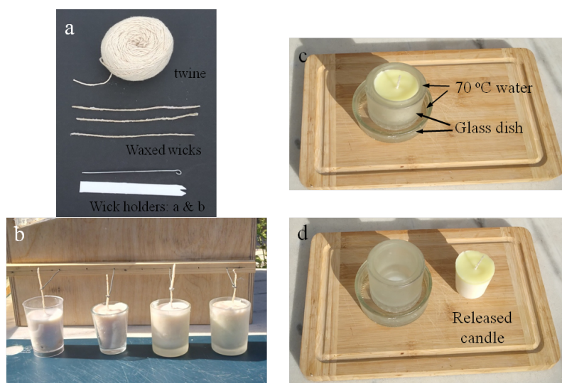
Figure 6. Photographs of wax re-casting and candle release process. (a) Kitchen cotton twine ball, waxed twine, and wick holders; (b) Poured mixed-wax into polycarbonate and glass molds of different shapes; (c) Post wax pouring. A 50 g blended wax candle within its glass mold is placed in 70–75 °C dual-water bath; (d) Blended-wax candle removed from its glass mold after approximately 45 s of treatment in the dual-water bath.
