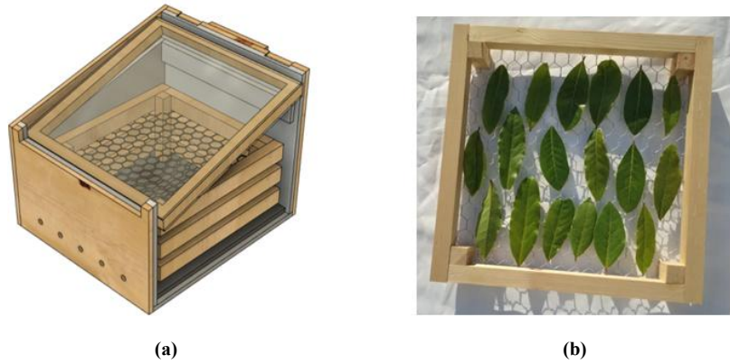
Figure 2. (a) 3D cross-section drawing of SBC-d; (b) Photograph of dehydration frame with three rows of 6 Bay leaves: total 18 leaves.
