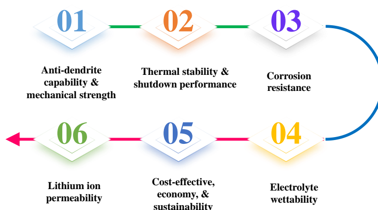
Figure 3. Detailed representation of separator performance prerequisites to contemplate when design the suitable separator for rechargeable LIBs.
