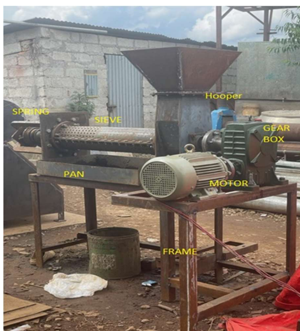
Figure 6. Fabrication of system.
