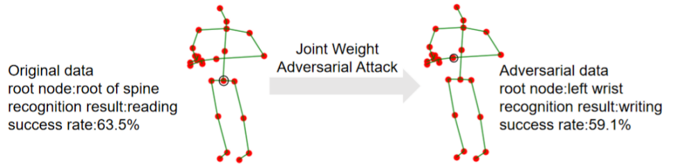
Figure 3. After the joint weight adversarial attack, the original data recognition result changed from 63.5% reading to 59.1% writing, and the root node changed from the root of the spine to the left wrist.
