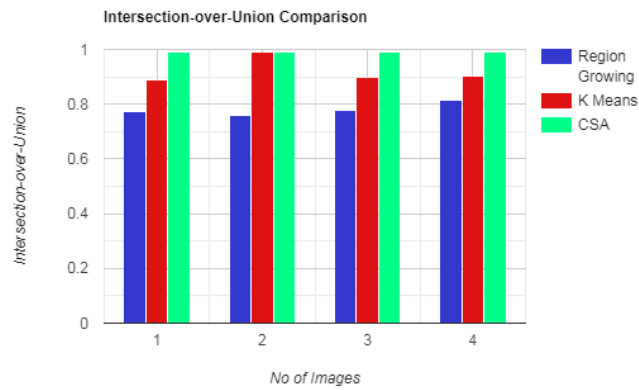
Figure 7. IoU of CSA, region growing and k-means clustering segmentation models.
