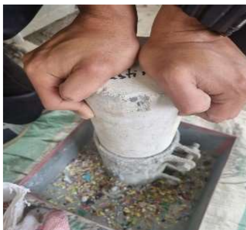
Figure 7. Compaction of LVPW.
