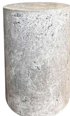
LVPW is slightly visible on the surface
