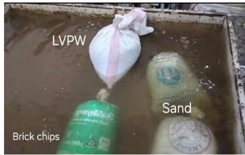
Figure 8. LVPW, sand & brick chips placed in water tank.
