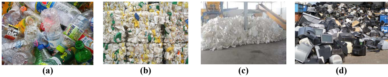
Figure 1. Wastes from (a) PET bottles; (b) HDPE waste; (c) expanded Polystyrene (EPS) foam; (d) electronic devices with plastic components.
